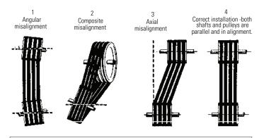
The modern wedge belt drive is a highly efficient power transmission medium, but optimum performance will not be achieved without correct tension and alignment.
